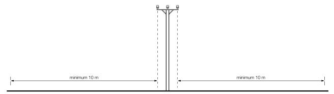
Figure 2 Minimum horizontal distances to overhead power lines
